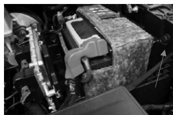
Figure 9- Ground Lug Connection
