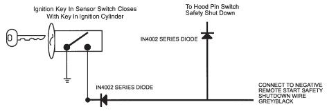
AFTER THE CONNECTION OF THE NEUTRAL START SAFETY WIRE AS INDICATED IN ANY OF THE PREVIOUS ALTERNATE CONFIGURATIONS, THIS CIRCUIT MUST BE TESTED FOR OPERATION
