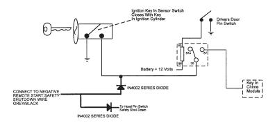
To connect to the key in sensor as shown in method 1:
