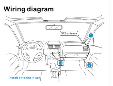
GPS antenna installation 1. Find a suitable mounting location. Clean the area with alcohol and use a strong double sided tape to attache the
