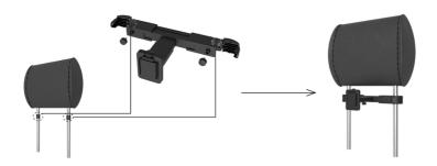
3. Plug in the harness cable into the monitor with the wires installed properly before docking it onto the headrest poles.
