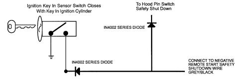
To connect to the key in sensor circuit as shown for method 2:
