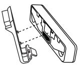
2. Push the Sound Bar down and back into the Sound Bar Bracket.
