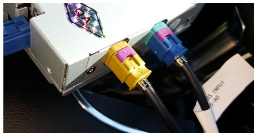
7. Mount the GPS antenna in a location so that it is not blocked by metal or glass containing a metallic coating. Route the GPS antenna to the Navigation Interface Module and connect to the BLUE Navigation antenna connector.
