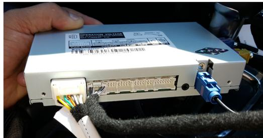
6. Route the YELLOW and BLUE video cables to the Navigation Interface's mounting location and connect to the Navigation Interface as shown.
