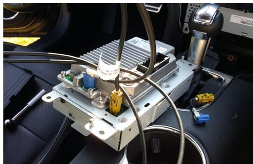
5. Route the main wiring harness to the Navigation Module's mounting location and connect the wiring harness to the Navigation Interface Module as shown.
