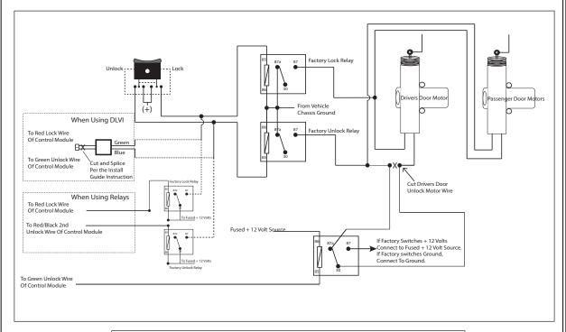
Resistive Circuits, As Well As 4 Wire Polarity Reversal and 5 Wire Alternating 12 Volt Door Lock Control Circuits
