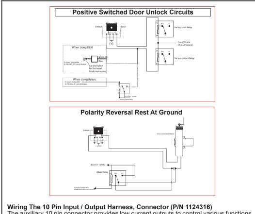
The auxiliary 10 pin connector provides low current outputs to control various functions in the vehicle during different stages of the Remote Start unit's operation. Understanding these outputs and the time in which they occur will allow you to determine if they are needed for the particular vehicle you are working on as well as how to use them.
