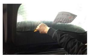
8. Disengage the clips, and remove the left and right side trim panels around the rear window.
