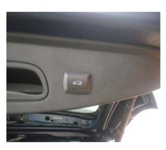
20. Mount the other open/close button in the driver's side lower dash panel as shown.
