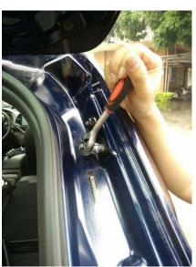
4. Install the supplied brackets to replace the OEM brackets, previously removed. Note the Left and Right side markings on the brackets for correct orientation.
