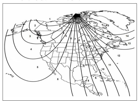
a) The zone setting is factory preset to Zone 8. Refer to Compass Calibration Zone Map to find correct compass zone setting for your geographical location. (Fig. 27)
