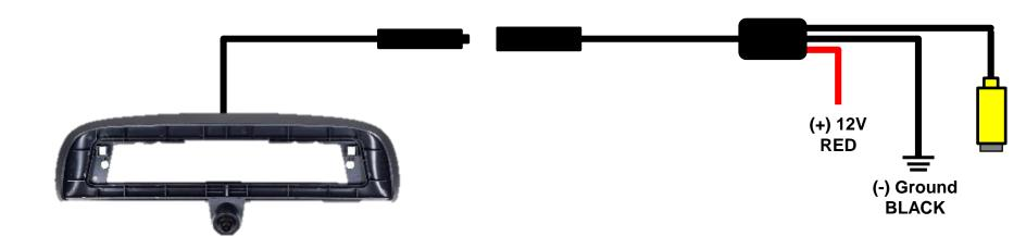
RED WIRE: Connect to 12V+ power source (ACC or IGN or REVERSE)
