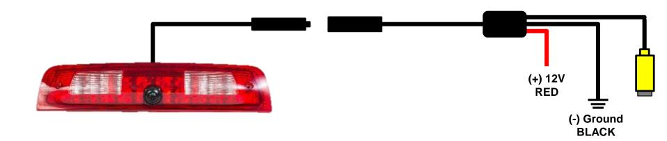
RED WIRE: Connect to 12V+ power source (ACC or IGN or REVERSE)
