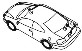
When mounting the camera make sure the surface in clean and oil free. Use the supplied angle wedges to adjust the sensor angle if needed. If the unit falses (beeps with no obstruction) adjust the angle upward away from the ground.
